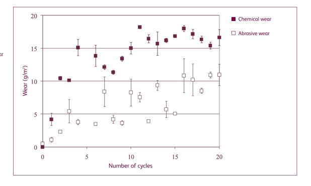
**Figure 3.0** Gloss of the tiles after the hydrofluoric treatment (■) and the abrasive wear  $(\Box)$ as a function of the number of cycles of hydrofluoric acid treatment and wear.
