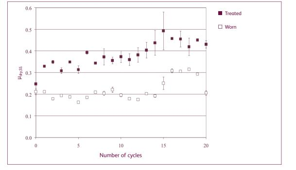
Surface properties and slip resistance of glazed ceramic tiles over-treated, or treated multiple times, with hydrofluoric acid
