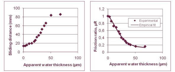
Figure 1.0 Example of the analysis of data generated by the Falling Plate Method.
