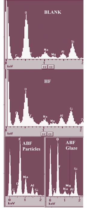
composition of the smooth glaze is almost the same as that of the BLANK tile. However, the composition of the submicron particles is quite different. They are mainly composed of F, Na, Mg, Al with very little SiO<sub>2</sub>. Since there is almost no fluorine atom on the original glaze, these results strongly suggest that the submicron particles originate from ammonium bifluoride which contains fluorine (NH<sub>4</sub>HF<sub>2</sub>). This explains the mass increase following the ABF treatment.
