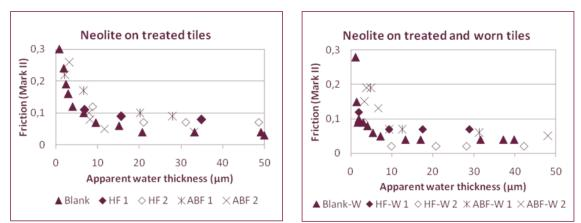
Tile numbers only distinguish independent data sets. Results obtained on the treated tiles (left) are compared with those obtained on the worn tiles (right). Results for the HF and HF-W were obtained with a solution of sodium lauryl sulphate (SLS) at 0.15% in water.
